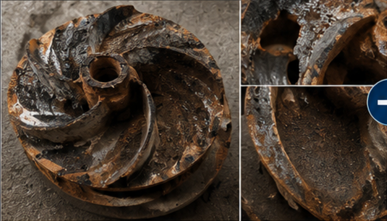
Severe corrosion, pitting, cavitation damage and material loss.
